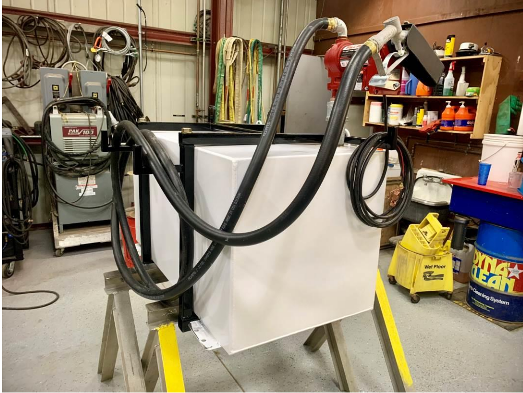
Above: Portable fuel tank fabrication
