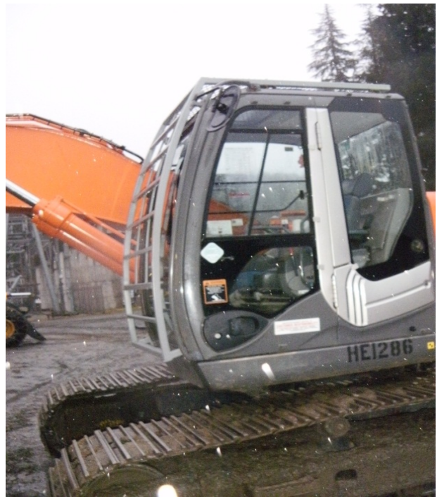
Excavator cab cage
