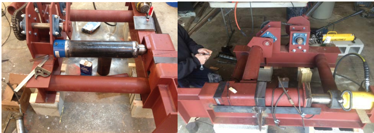
Full-scale model, placing the load cell (blue) to measure the resultant brace force from the friction block in the left photo; the kicker brace replaced and partially loaded in the right-hand photo above.
