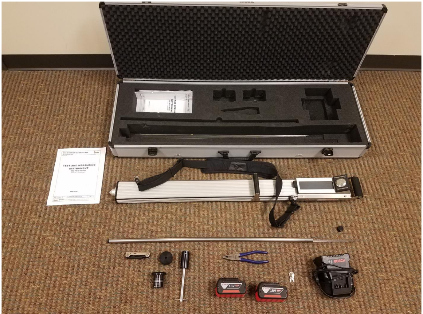
IML PD-600 Resistograph for Wood Pole Testing
