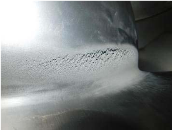
Runner cavitation frosting close-up
