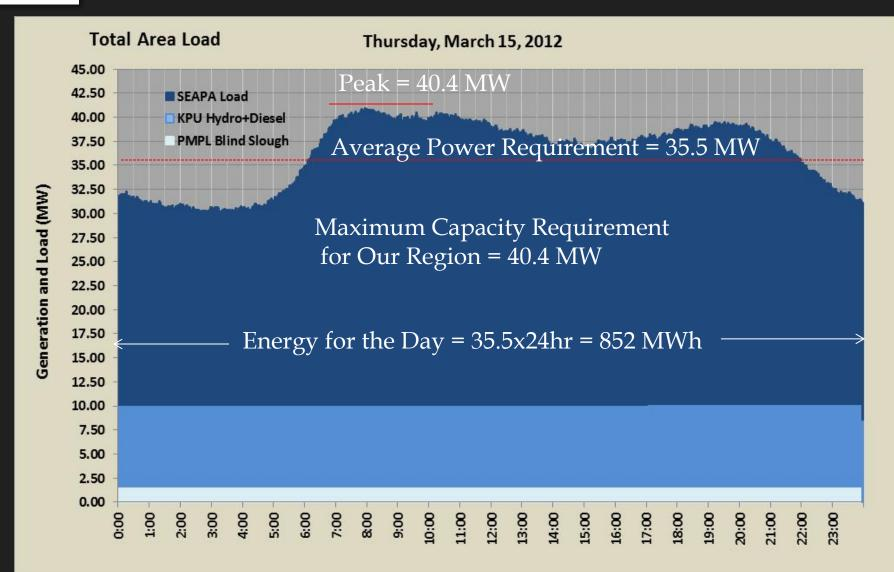
This is total load + distribution losses plus transmission and SEAPA plant consumption
