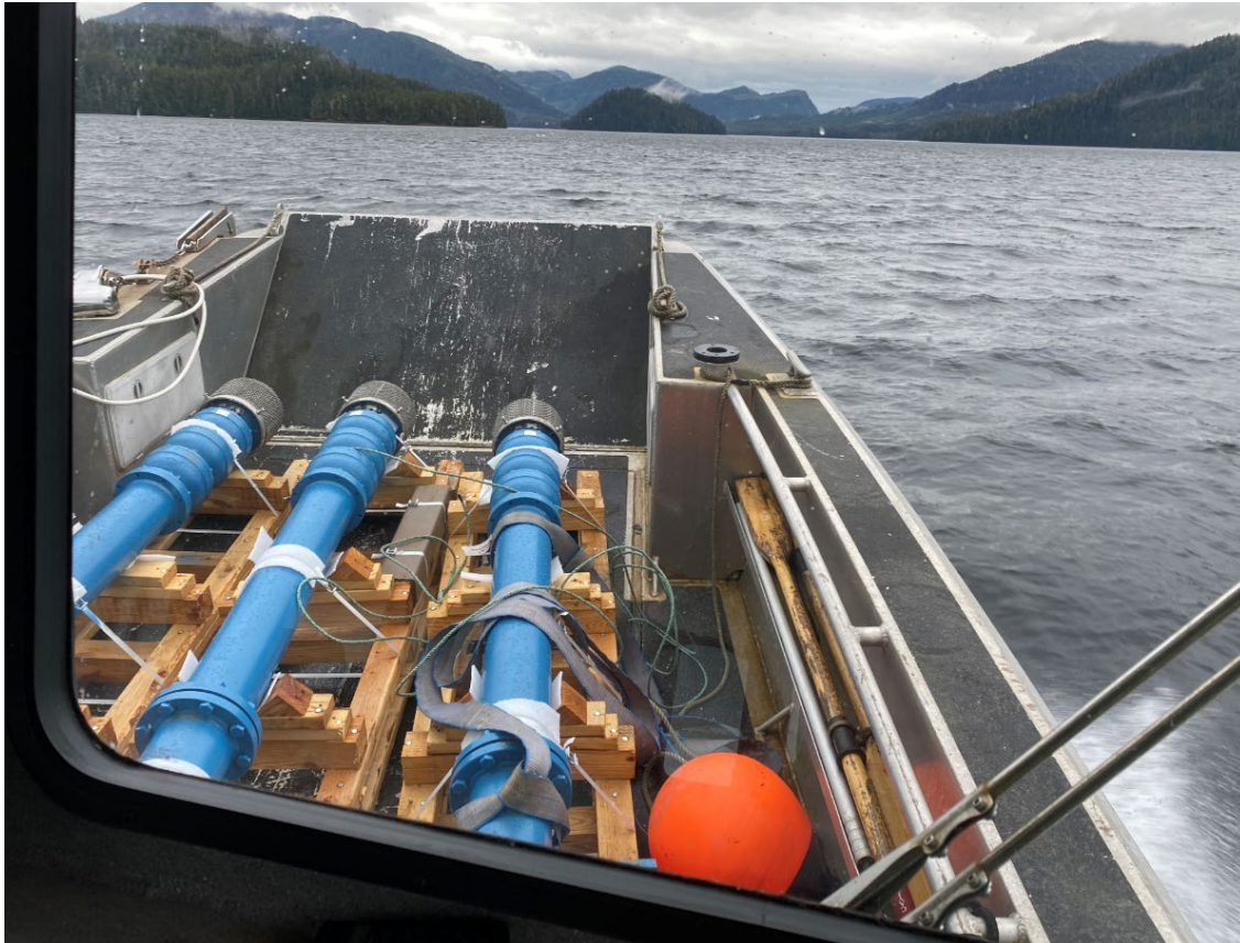
Cooling Water Pumps on their way to Tyee
