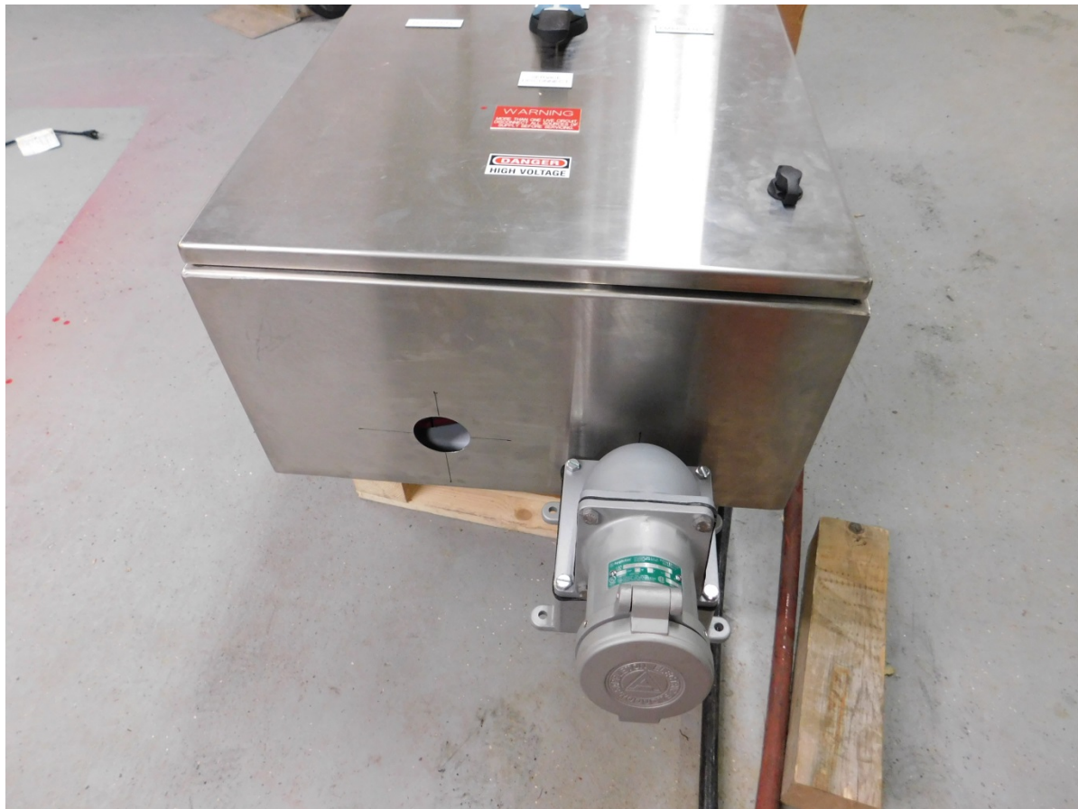
Below: Fabrication of Emergency Generator Transfer Switch & connection port
