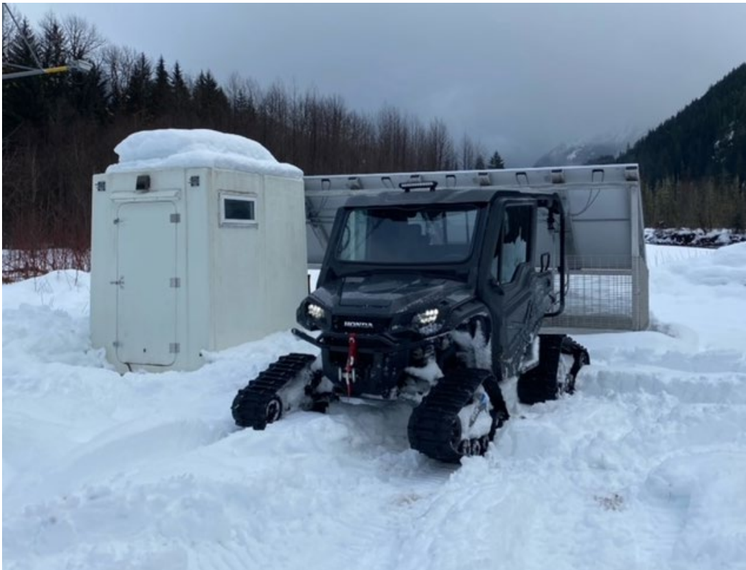
Track Kit installed on Honda side-by-side for access to Communication SAT pads.
