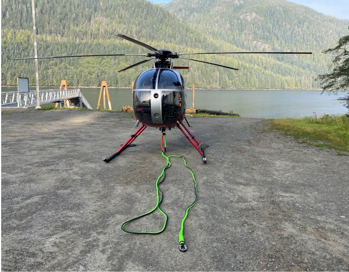
Figure #6 - TEMSCO helicopter rigged with new 50' short haul line rated for External Human Cargo
